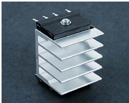
Q-Pad II is a composite of aluminum foil coated on both sides with thermally / electrically conductive Sil-Pad rubber. The material is designed for those applications in which maximum heat transfer is needed and electrical isolation is not required. Q-Pad II is the ideal thermal interface material to replace messy thermal grease compounds.
