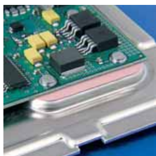
Here, Sil-Pad 900S enhances the thermal transfer from this FR-4 circuit board with thermal vias to the metal base plate.
