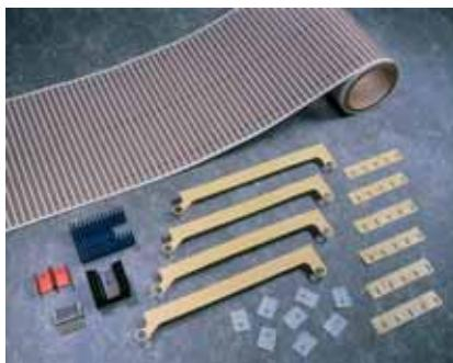
Poly-Pad K-10 is a composite of film coated with a polyester resin. The material offers superior thermal performance for your most critical applications with thermal resistance of 0.2°C-in<sup>2</sup>/W as well as excellent dielectric strength.
