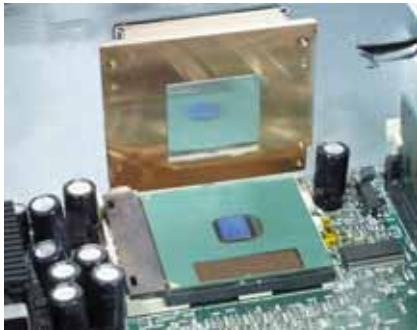
Bergquist's reworkable Hi-Flow 225UF thermal interface material provides a low thermal resistance path between hot components such as high-performance processors and heat sinks.
