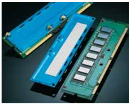
Gap Pad HC 1000 is an extremely conformable, low-modulus polymer that acts as a thermal interface and electrical insulator between electronic components and heat sinks. The "gel-like" modulus allows this material to fill air gaps to enhance the thermal performance of electronic systems. Gap Pad HC1000 is offered with removable protective liners on both sides of the material.
