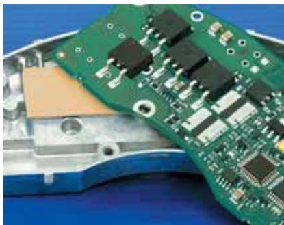
Gap Pad A3000 is a thermally conductive, filled-polymer laminate, supplied on a reinforcing mesh for added electrical isolation, easy material handling and enhanced puncture, shear and tear resistance. Gap Pad A3000 has a reinforcement layer on the dark gold side of the material that assists in burn-in and rework processes while the light gold and soft side of the material allows for added compliance.
