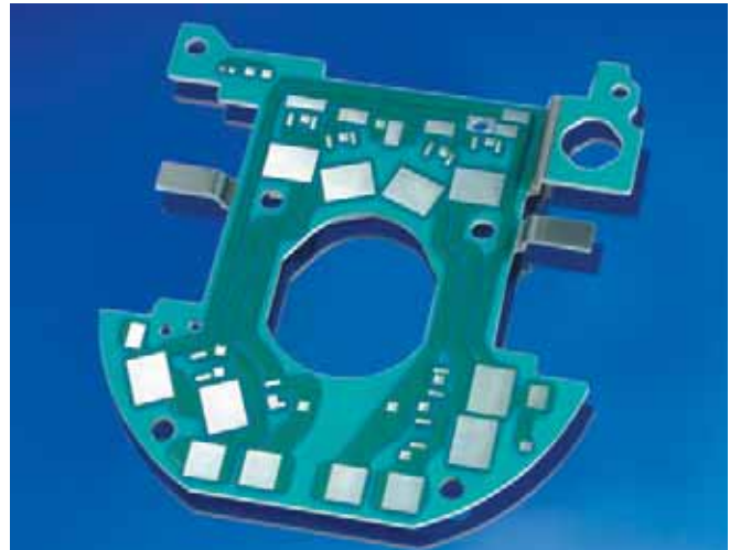
Thermal Clad is a versatile substrate. In this motor control application, the dielectric has been selectively removed and the metal has been formed with three-dimensional features.
